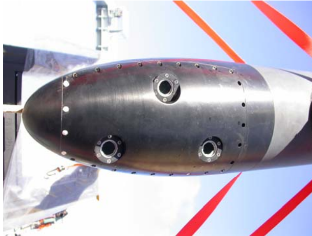
Figure 3: An underwater DDPIV system with a shortened aperture layout to reduce drag.
